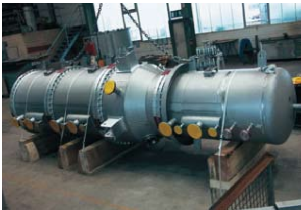
3-stages overhead condenser
