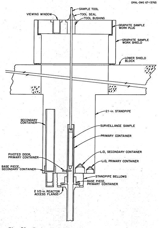
Fig. 25. Equipment for Handling the Surveillance Sample.
