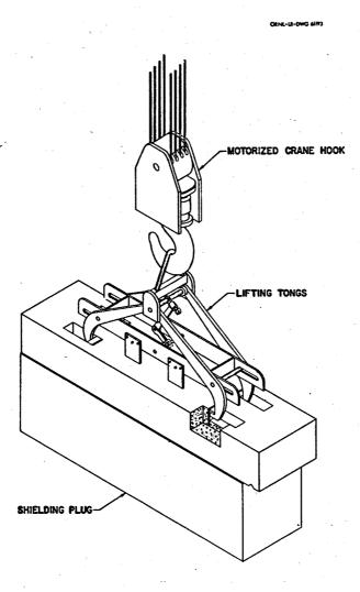
Fig. 3. Remotely Operated Lifting Tongs for Shielding Plugs.
