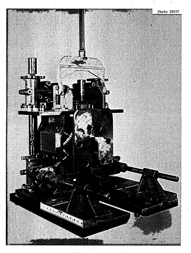
Fig. 18. Positioning Vise for Remote Brazing.
