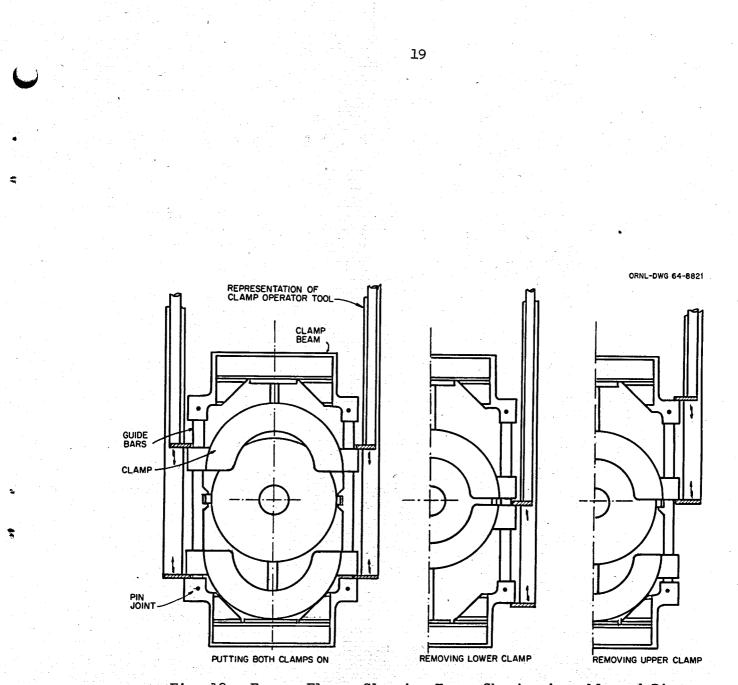
Fig. 10. Freeze Flange Clamping Frame Showing Assembly and Disassembly Steps. the motion is precisely controlled until the entire weight of the flange clamp assembly is carried by the tool. The assembly is then moved horizontally back along the piping and hung on the clamp stowing bracket, as shown in Figs. 9 and 11.
