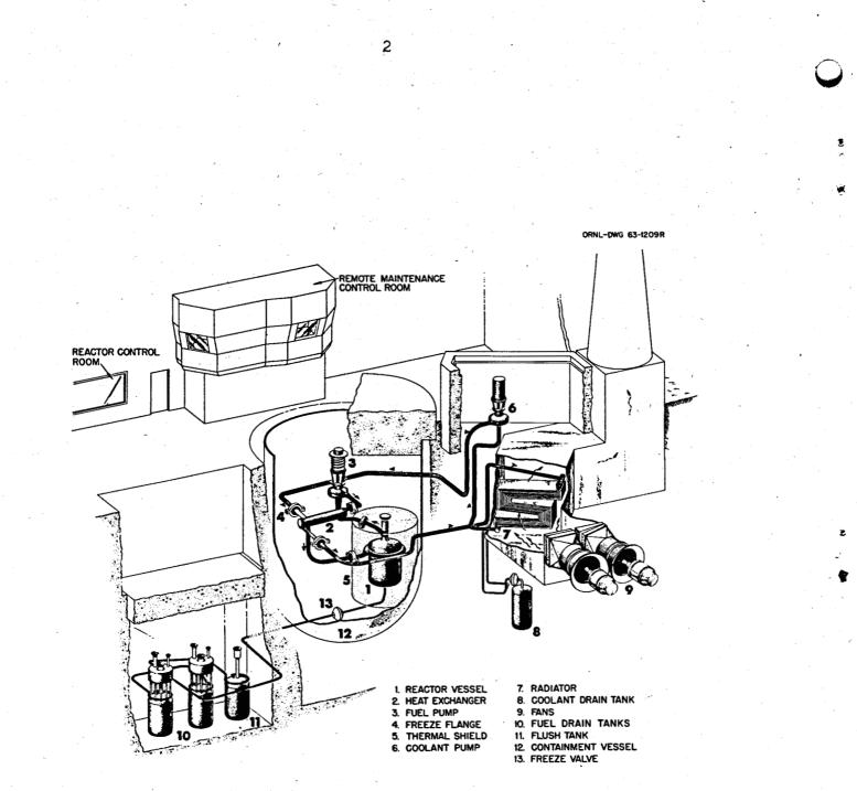
Fig. 1. Sketch of MSRE Arrangement and Flow Diagram.
