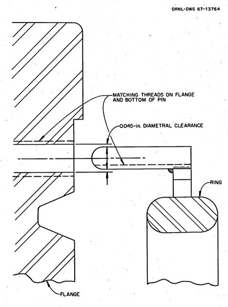
Fig. 12. Detail of Arrangement for Locking Ring to Flange During Maintenance.
