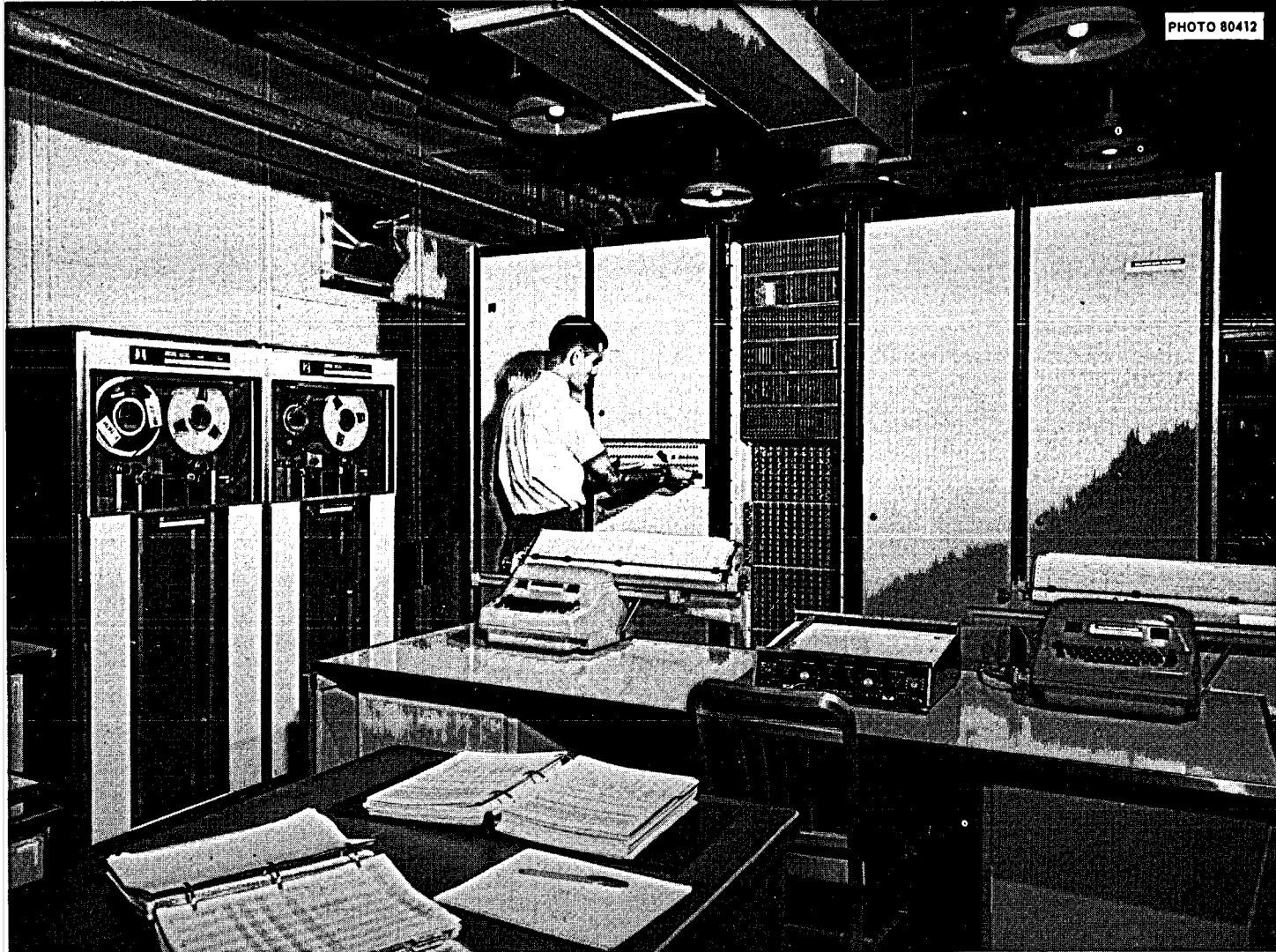
Fig. 2.12.2. Bunker-Ramo 340 Computer Central Processor.
