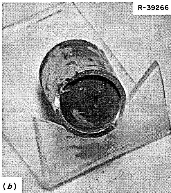
Fig. 6.6. Surface appearance of fuel salt before and after beryllium exposure to ^{235}\text{U} fuel salt. (a) FP-12-55, (b) FP-12-57. Salt analyses did not reflect significant differences in chromium concentration nor were they indicative of the identity of the material at the blackened surface.
