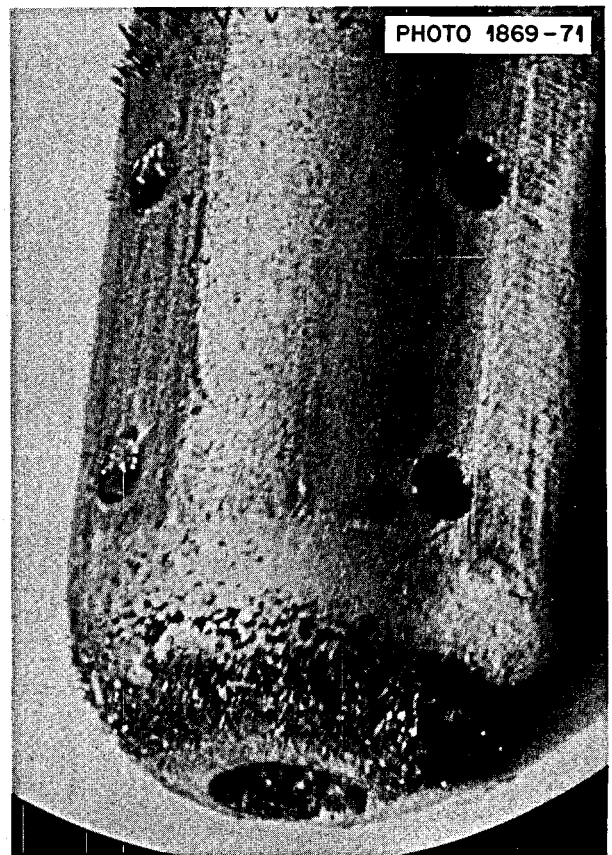
Fig. 6.13. Metallic particles on copper capsule used to expose a magnet to ^{233}\text{U} fuel salt. November 15, 1968, FP-15-61. Dendrites on capsule were composed of fine particles of iron.
