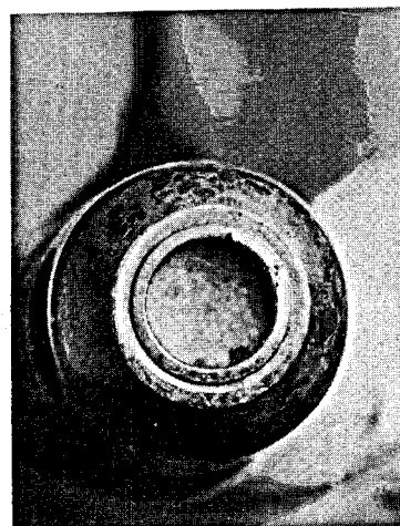
FP 19-25 CAPSULE VIEWED FROM BOTTOM, SHOWING SALT RESIDUE IN CAPSULE.
